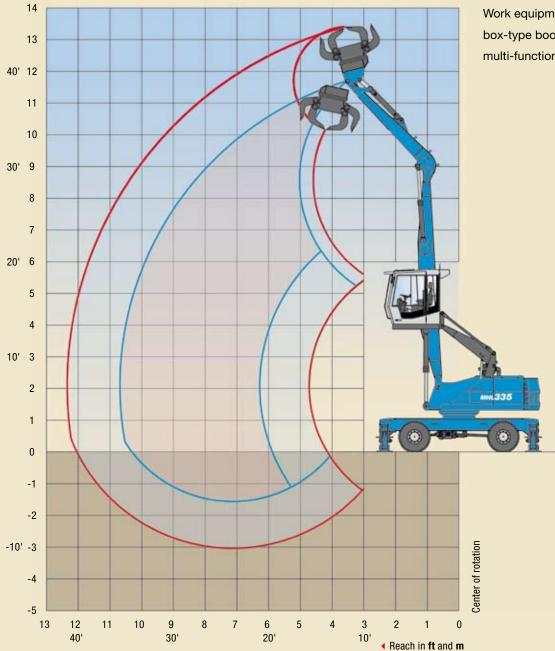
Work equipment: box-type boom 21.3' (6.5 m), multi-function stick 13.1' (4.0 m)
